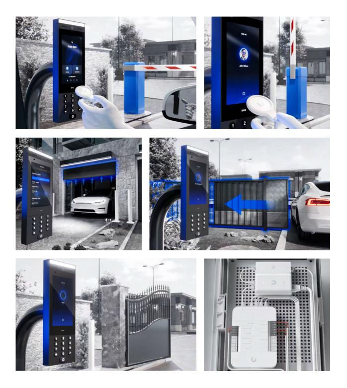
Ubiquiti's UniFi Access represents a cutting-edge access control system driven by native Power over Ethernet (PoE) technology. This system accommodates traditional electric bolts, magnetic locks, and various 12V access peripherals like motion sensors, push buttons and alarms.
